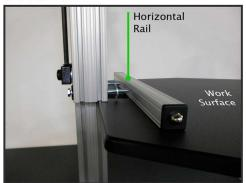
Step 8: Lift the Work Surface up and align the holes in the Horizontal Rail with the (2) 1/4-20 x 3.50 Hex Head Bolts. Push the Work Surface onto the Hex Head Bolts until the threads of the bolts
