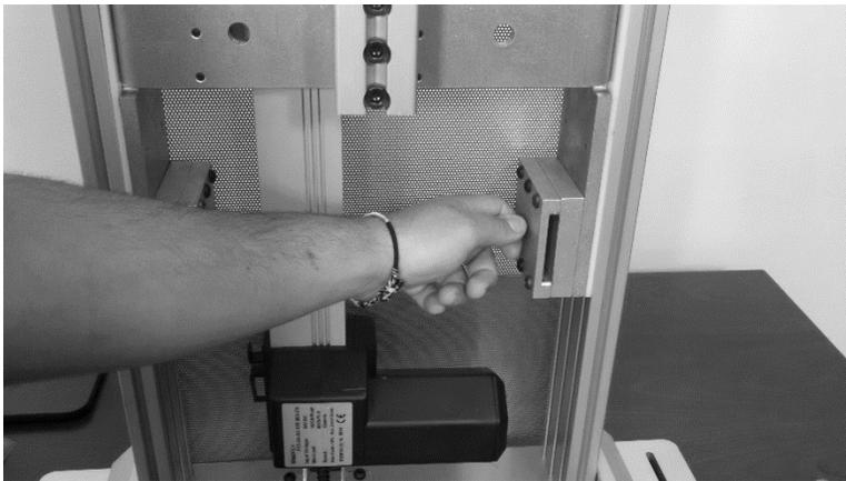
*Loosen the screws in the middle of the work surface support brackets as shown.*
