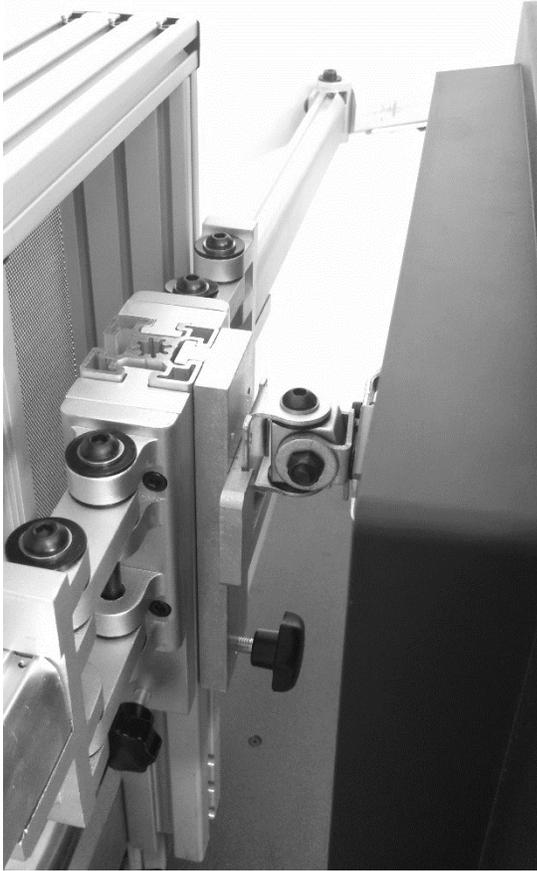
*To install right and left pivots, tilt monitor back and place hook over monitor arms. Bring the monitor forward to secure. To remove the monitor, pull up on the knob while tilting the monitor back.*
