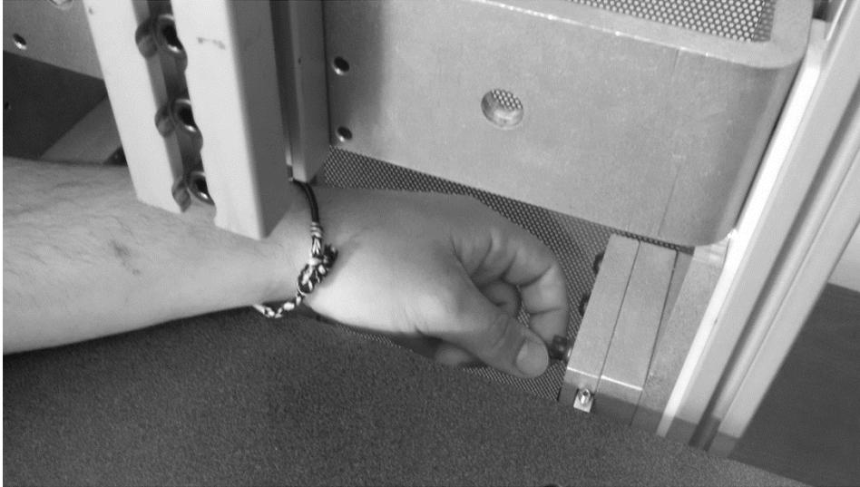
*Hand tighten the thumb screws fully to secure the work surface.*
