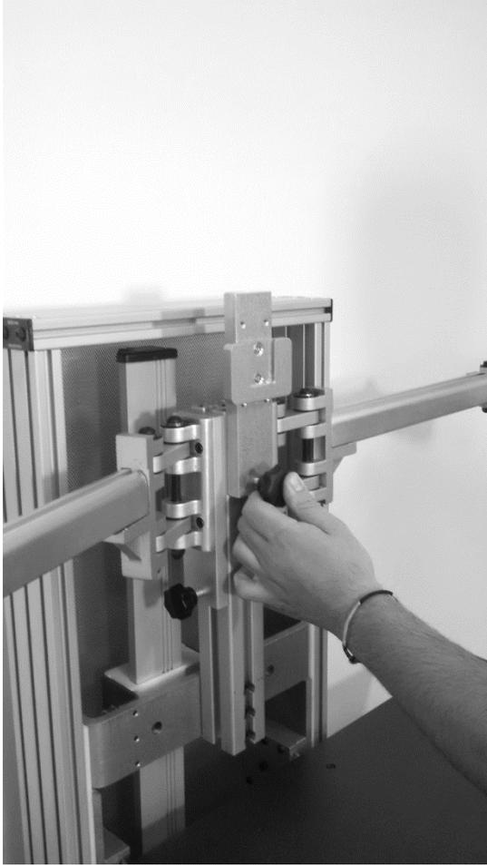
*If a center monitor is required, slide the center monitor mount in the vertical post and secure with the plastic knob.*
