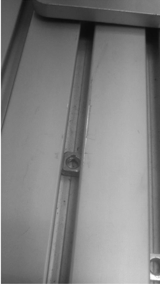
*If installing unit to a flush rail, drop the square nuts in T channel and line them up with the slots on the baseplate of the unit.*
