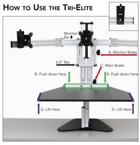
To move the mount horizontally closer or farther apart, simply loosen the bolt attached to the horizontal monitor rail (B) by a single turn with a 5/32 allen wrench. Once you have reached the desired position tighten the bolt.
