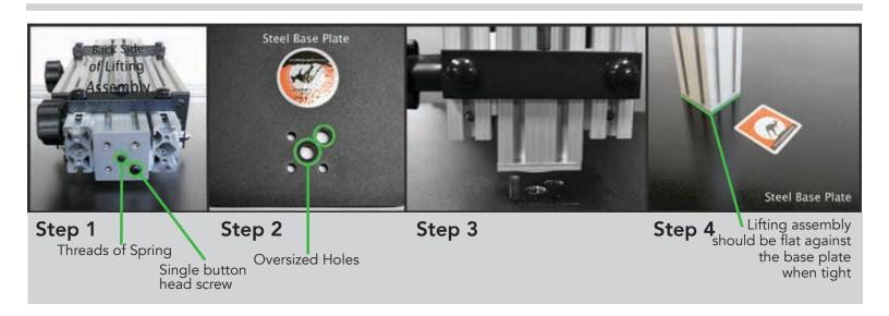
**Step 1:** Lay the lifting assembly on a solid surface with the back side up as shown. Notice the single Button Head Bolt in the assembly union plate. **DO NOT LOOSEN THE SINGLE BUTTON HEAD BOLT THAT IS NOTATED.**
