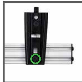
To move the mount horizontally closer or farther apart, simply loosen the bolt attached to the horizontal monitor rail (D) by a single turn with an 5/32 allen wrench. Once you have reached the desired position tighten the bolt.
