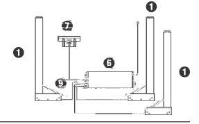
**M.** Turn the assembled desk right-side-up. With two people grab the desk by the base (not the desktop) and turn the desk right-side-up. Adjust the Leveling Studs (Part #8) on the Feet (Part #2) as needed.
