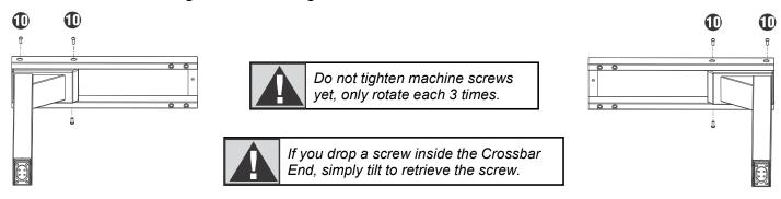
C. IMPORTANT! DO NOT TIGHTEN SCREWS IN THIS STEP, ONLY INSERT THEM AND ROTATE 3 TIMES. YOU WILL TIGHTEN IN STEP D.
