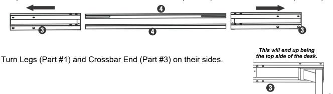
B. IMPORTANT! DO NOT TIGHTEN SCREWS IN THIS STEP, ONLY INSERT THEM AND ROTATE 3 TIMES. YOU WILL TIGHTEN IN STEP D.
