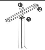
**G.** Your desktop may or may not be pre-drilled. Please check both sides of the desktop before placing the desk base on it for pre-drilling! Carefully place the upside down desk base on the underside of the desktop.
