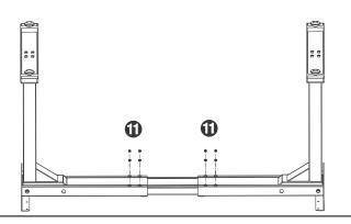
I. Double-check that the base is centered on the underside of the desktop and is located where you want it. Also, double-check that the included wood screws are not too long for your desktop and screwed all the way in.
